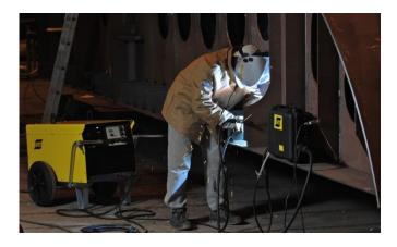
The welding properties of these units are configured to meet the requirements of welding with celluloid electrodes. The arc is very flexible when starting from the lowest currents.
