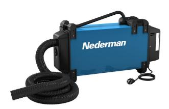
The Fume Eliminator 840 is designed to be carried to the working area. Connected to a an extraction nozzle or a welding torch, the FE unit extracts the fume directly at source. The FE 840 has a manual start/stop function and is suitable for extraction of fume from maintenance welding applications.
