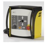
With control panel on the front Suitable for ESAB's A2 / A6 tractor automats and A2 / A6 beam travelling carriage. Automatic solutions with short distance between welding head and GMH control box and where the operator has a good overview of weld joint and welding head without moving around.
