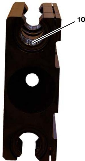
The linear bearings of the slide consist of two steel shafts (4) and four ball bushings (10).
