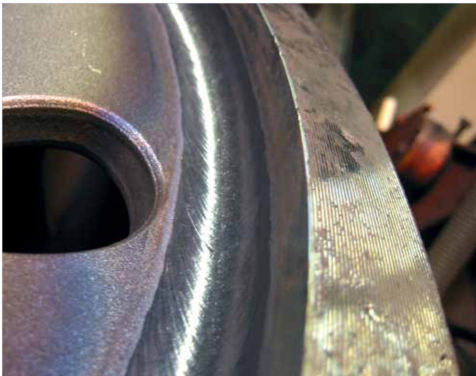
Downhand (PA/1F) fillet weld showing perfect wetting and smooth finish.
