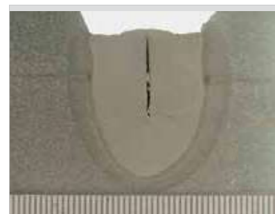
Weld depth to width ratio > 1 and relatively large amount of impurities in base material (S, P, Nb).
