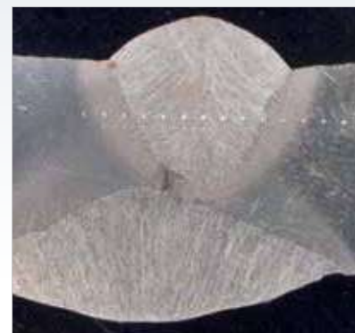
Insufficient penetration and excessive reinforcement; also misaligned.
