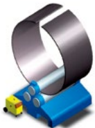
Rolling, forming and tack welding of the shell
